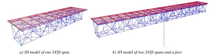
Figure 3. 3D models used for analyses of the south approach superstructure.
