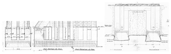
Figure 5. Foundations for Piers 24 (left) and 25 (right).
