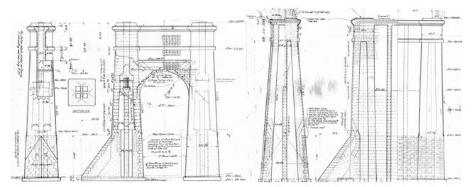
Figure 4. Piers 23 (left, 26 similar) and 24 (right, 25 similar) elevations showing hollow section.
