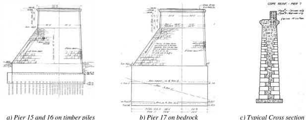
a) Pier 15 and 16 on timber piles
