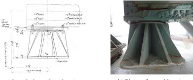
a) Details from shop drawings b) Photo of actual bearing Figure 8. – Spherical bearings on Jacques-Cartier bridge.
